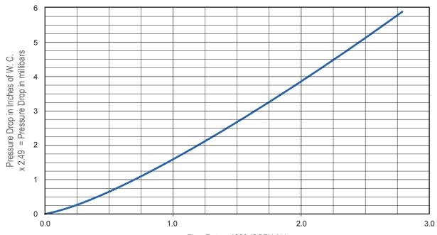
Flow Rate x 1000 (SCFH Air) x 0.472 = Flow Rate in Cubic Meters Air/ Minute
