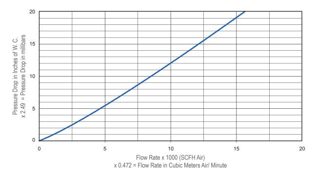
Flow Curves 59 IN-LINE DETONATION ARRESTER (Model 59-004)
