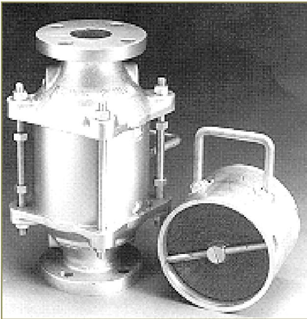
Two pieces are shown on the photo (shown left). The left is the entire unit, and the right piece is the core assembly. The core assembly is made of spiral-wound crimped ribbon susceptible to clogging. This core assembly is what stops the flame from propagating downstream of the ignition source.
