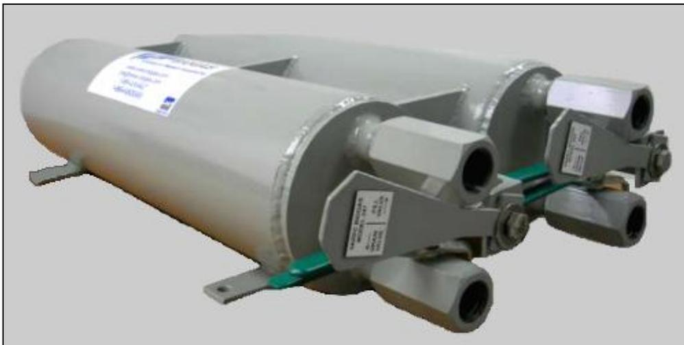
The Model 247D Low Profile High Pressure Drip Trap is rated for a maximum working pressure of 100 psig (688 kPa). This unit is typically installed at low points in the gas piping downstream of booster blowers or compressors. The 247D is ideal for blower and compressor skids because it can be installed low to the ground while providing a larger reservoir for condensate collection.
