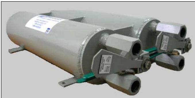
The Model 247D Low Profile High Pressure Drip Trap is also rated for a maximum working pressure of 100 psig (688 kPa). This unit is typically installed at low points in the gas piping downstream of booster blowers or compressors. It is ideal for tight or confined spaces in blower skid or compressor skids. It also provides for a larger reservoir capacity.
