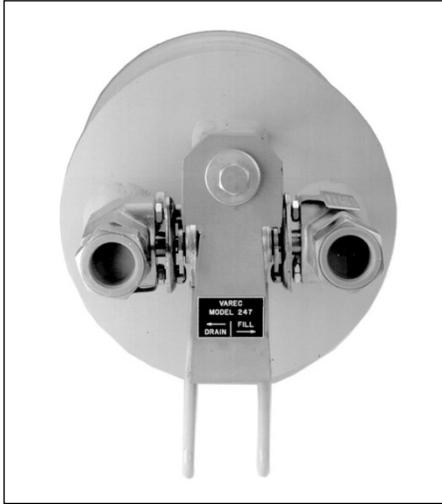
The Model 247 High Pressure Drip Trap is rated for a maximum working pressure of 100 psig (688 kPa). This unit is typically installed at low points in the gas piping downstream of booster blowers or compressors.
